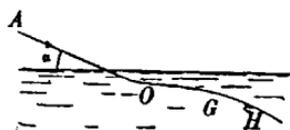
In these tests  $v_0 = 625.3$  m/sec. If  $\alpha = 7^\circ$ , the velocity of the projectile is diminished to such an extent by the resistance of the water, that it no longer rises to the surface, but continues to fall downwards along the path  $OGH$ .
